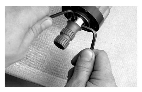
**8a.** Recentering: The set screws jack against the two flats or ramps on the torsion bar as shown in the cutaway views below:
